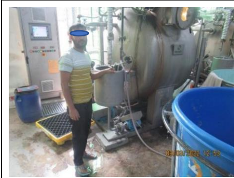
NC Picture 01: Dyeing section operators were not using respiratory mask, hand gloves
